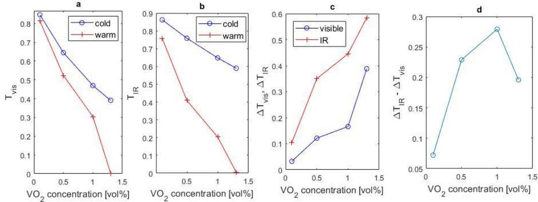
Figure 3: Impact of the VO<sub>2</sub> concentration in solar transmittances for both cold and warm states of the material, in the visible (a) and infrared region (b), their modulations between both states of the material (c) and difference between infrared and visible transmission modulations (d)
