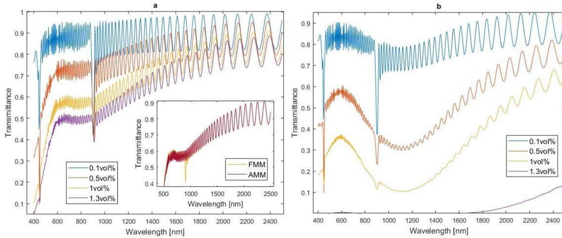
Fig. 2: Transmission spectra of the polymer opal loaded with different  $VO_2$  concentrations computed with FMM (a) in cold state (inset: comparison with an equivalent homogeneous material computed with AMM, in the case of 1vol%  $VO_2$ ) and (b) hot state
