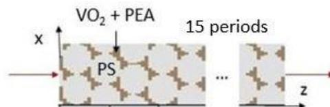
Fig. 1: Numerical representation of a close packed polymer opal made of PS spheres in PEA filled with VO<sub>2</sub> nanoparticles, and light incident over the (111) crystallographic direction
