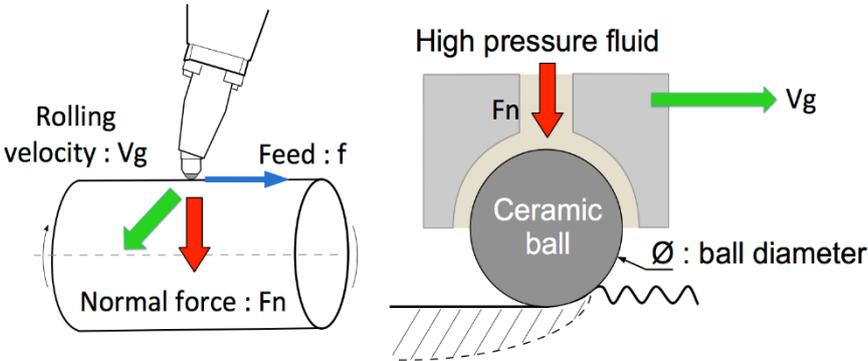
Figure 1 : Principle of the ball-burnishing process (reprinted from [29] with permission from Elsevier).
