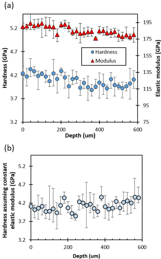
Figure 5 : (a) Hardness and elastic modulus in-depth profiles of the ball-burnished specimen ; (b) Hardness in-depth profile of the ball-burnished specimen computed from nanoindentation measurements considering a constant Young modulus (185 GPa)
