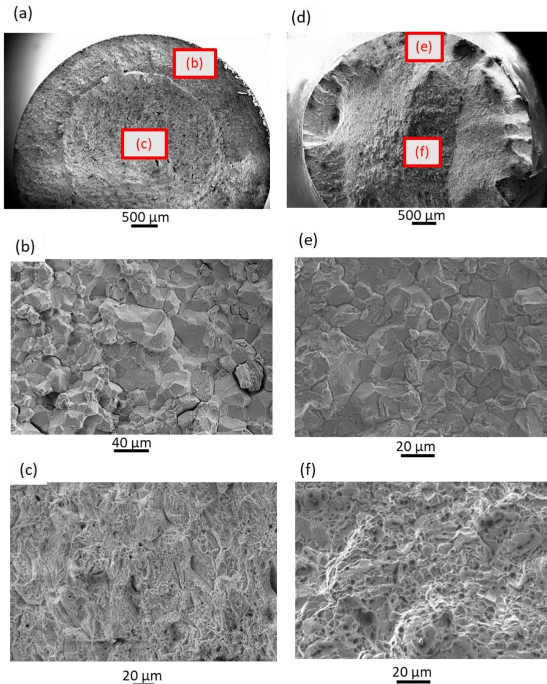
Figure 8 : Fracture surfaces after tensile test for the polished specimens (a-c) and the ball-burnished specimens (d-f) for the H charged,  $10^{-4}$  mm/s condition.
