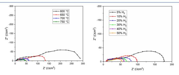
Figure 4. Nyquist plots of the full cell  $MnO_x/LSGF|LSGM|LSCF$  are reported as a function of temperature using 30% of hydrogen (left) and as a function of hydrogen content at 700 °C (right).
