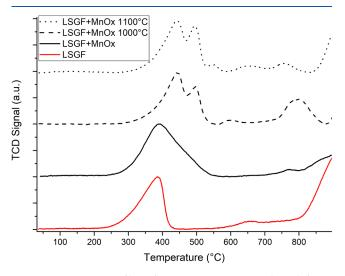
Figure 2.  $H_2$ -TPR profiles of LSGF + MnO<sub>x</sub> treated at different temperatures. In red, the profile of LSGF before the deposition is shown for comparison.
