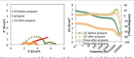
Figure 7. Comparison between impedance spectra before, during, and after propane feeding. Left: Nyquist plots. Right: Bode plots.
