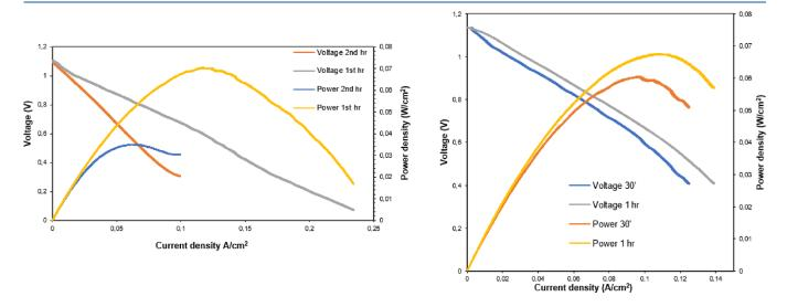
**Figure 6.** Left: cell polarization curves after switch-on (first hour) and after 1 h of operation (second hour) at 744  $^{\circ}$ C. The anode is fed with pure H<sub>2</sub>, 53 sccm. Right: polarization curves and power of the cell fed with propane at the anode. Results after 30 min and 1 h of operation are reported. The temperature is 744  $^{\circ}$ C, and the gas flow at the anode is 50 sccm. In both cells, the cathode was fed by air.
