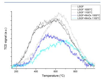
**Figure 3.** O<sub>2</sub> desorption of the tested samples. O<sub>2</sub>-TPD profiles of LSGF and LSGF +  $MnO_x$  treated at different temperatures. The profile of LSGF treated at 900 °C for the calcination is represented by the dashed line.
