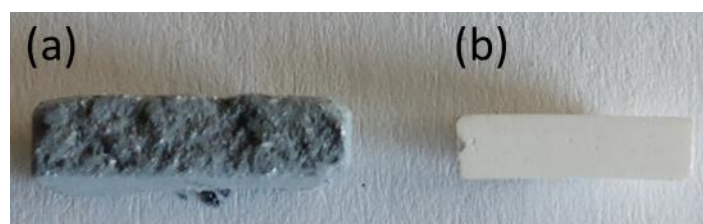
Figure 7: Cross-section of the C B HA-C-900-H60 pellet (a) before and (b) after sintering
