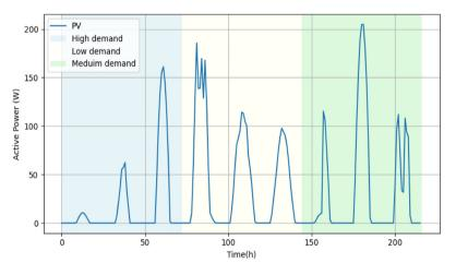
Fig. 4. Profile of one  $m^2$  of PVs for nine typical days from three seasons (high = winter, low = summer, medium = spring) simulated using HelioScope solar design software.
