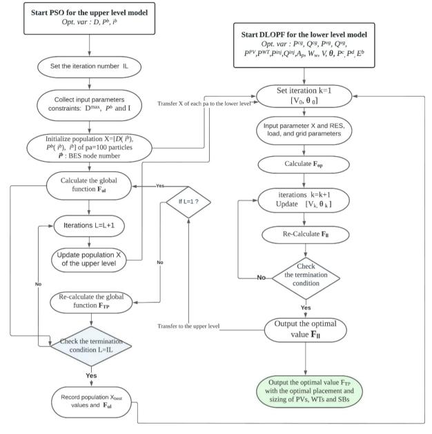
Fig. 1. Flowchart for the proposed bi-level PSO-DLOPF solution.
