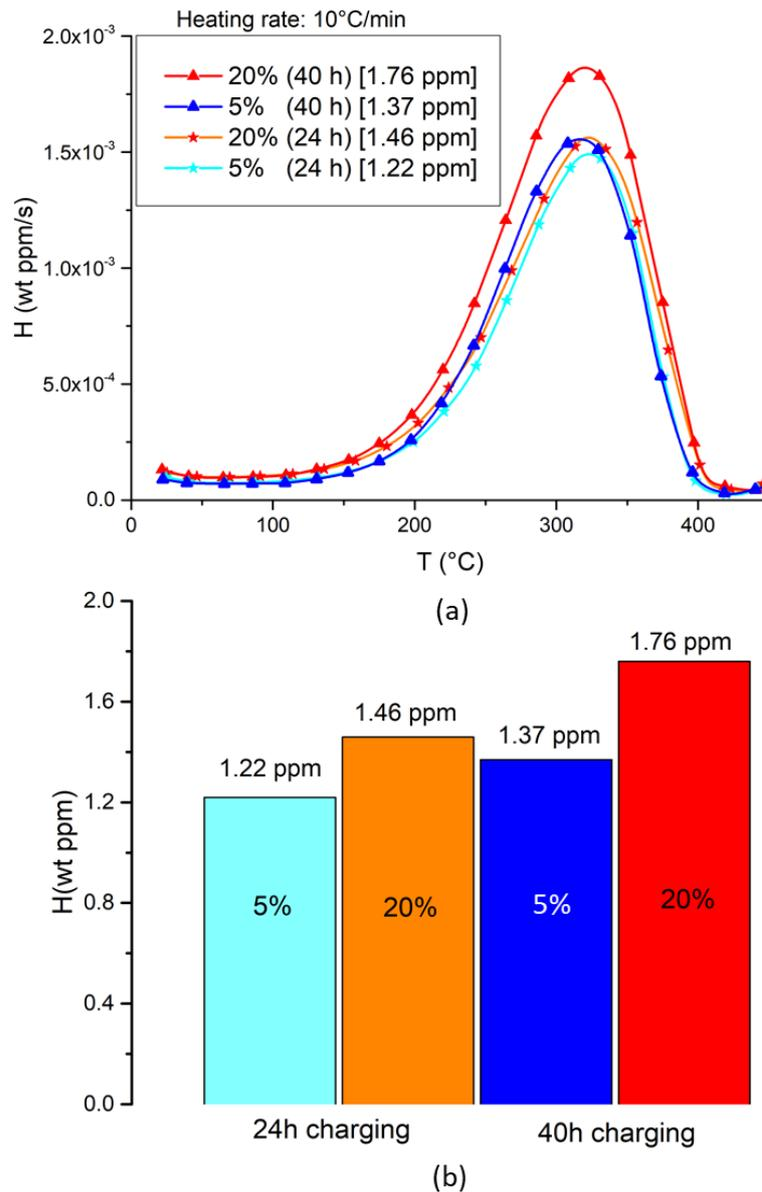
Figure 9 : The influence of the immersion time on the amount of absorbed hydrogen for two different  $\text{NH}_4\text{SCN}$  concentrations (5 wt% solution and 20 wt% solution) (a) TDS spectrums; heating rate = 10°C/min (b) Hydrogen content as a function of the charging solution concentration. The hydrogen content was evaluated from TDS peak integration. The same sample was used for all the experiments.
