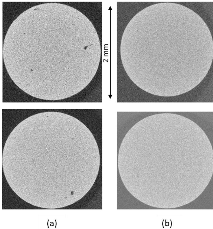
Figure 1 : Cross sectional views of (a) a cast sample (b) a forged sample based on X-ray tomography data, showing a few cavities in the cast sample and the absence of porosity in the forged sample.
