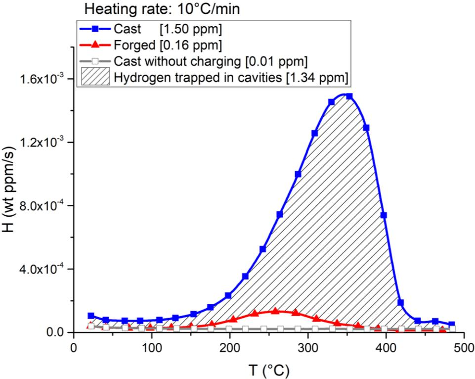
Figure 10 : TDS spectra for a cast sample without charging, a charged cast sample and a charged forged sample. The charging was performed in a 5 wt% NH<sub>4</sub>SCN aqueous solution for 24 h charging. The heating rate was 10°C/min. The cast sample has a volume fraction of porosity of 0.27%.
