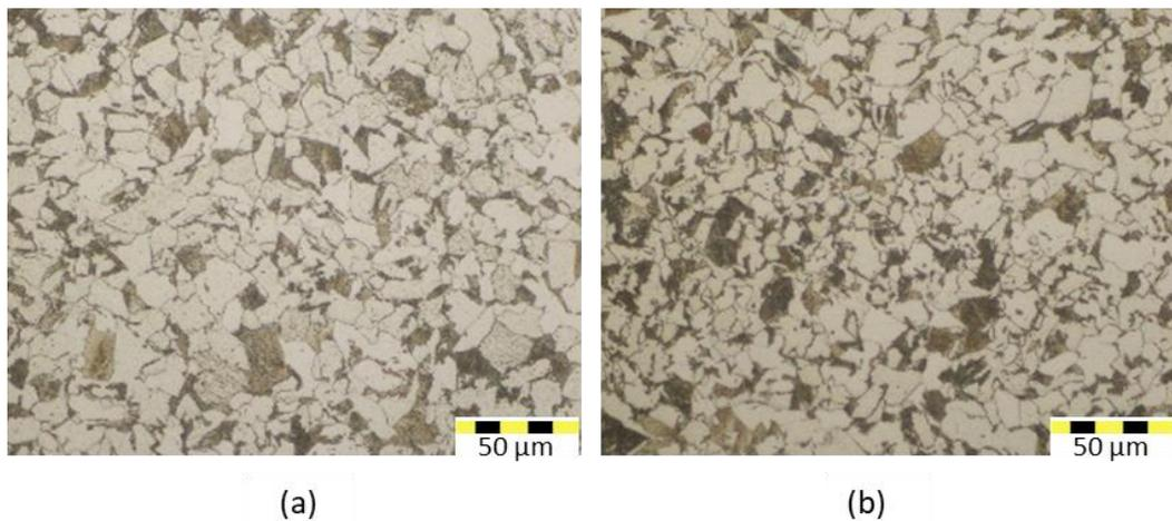
Figure 4 : Optical micrographs of etched (a) cast sample and (b) forged sample showing a ferritic-pearlitic microstructure. The micrographs were taken from regions of the specimen showing no porosity.
