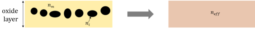
Figure 2: Schematic representation of a heterogeneous oxide layer modeling by computing a homogeneous effective refractive index through the Maxwell-Garnett approximation.
