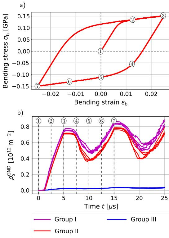
**Fig. 7.** CDD simulation of bi-directional bending. (a): Cycle of bending moment based on the displacement driven loading. For the definition of the bending stress and strain, see Eqs. (11) and (12). (b): Resulting GND density evolution for the 12 different slip systems grouped according to Sec. 2.
