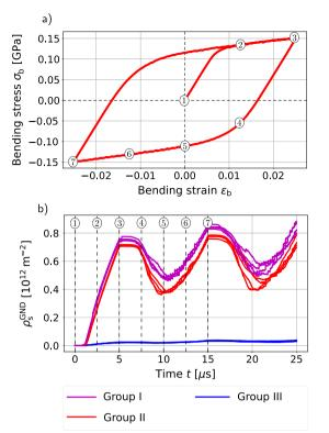
**Fig. 7.** CDD simulation of bi-directional bending. (a): Cycle of bending moment based on the displacement driven loading. For the definition of the bending stress and strain, see Eqs. (11) and (12). (b): Resulting GND density evolution for the 12 different slip systems grouped according to Sec. 2.
