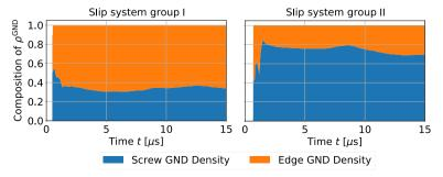
Fig. 8. Comparison of the composition of the screw and edge dislocation density for the active slip system groups over the microstructure evolution.
