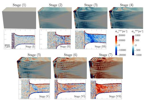
**Fig. 10.** Evolution states of  $\alpha_{13}$  over the loading stages 1-7 (according to Fig. 3.)
