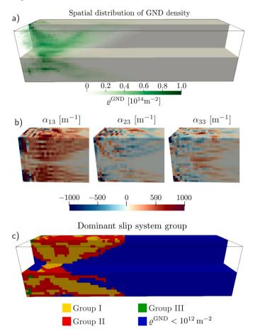
**Fig. 9.** Distribution of GNDs at stage 7 of the CDD simulations. (a): The spatial distribution of the GND density, (b): contour plots of the tensor components  $\alpha_{i3}$  and (c): the dominant slip system groups over the cantilever beam.
