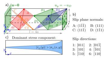
**Fig. 1.** a) Considered system geometry and the slip planes of the FCC sample. b) Specific vectors corresponding to the slip planes and the BVs. c) The schematics highlights with blue the region on the front face of the cantilever where the shear stresses are larger than the compressive stresses.
