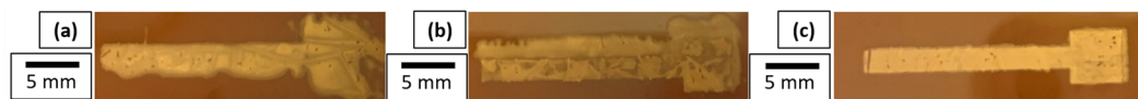
Figure 15. Pictures of (a) 40 layers of coating printed 20 layers by 20 layers; (b) 40 layers of coating printed 10 layers by 10 layers; and (c) 60 layers of coating printed 5 layers by 5 layers onto PI foils of a 2.5 cm length pattern printed.
