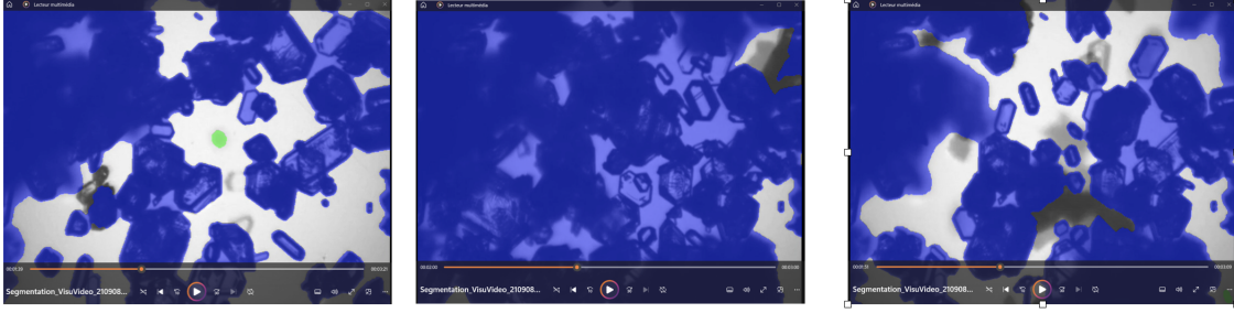
Fig 9 Critical cases with excessive air gap clogging result in poor segmentation of the glued part and a spatial support too constrained for accurate moving aggregate detection.
