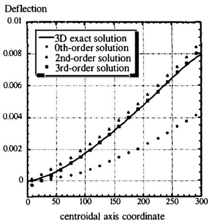
**Fig. 3 Deflection of the cantilever beam**
