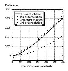
Fig. 3 Deflection of the cantilever beam
