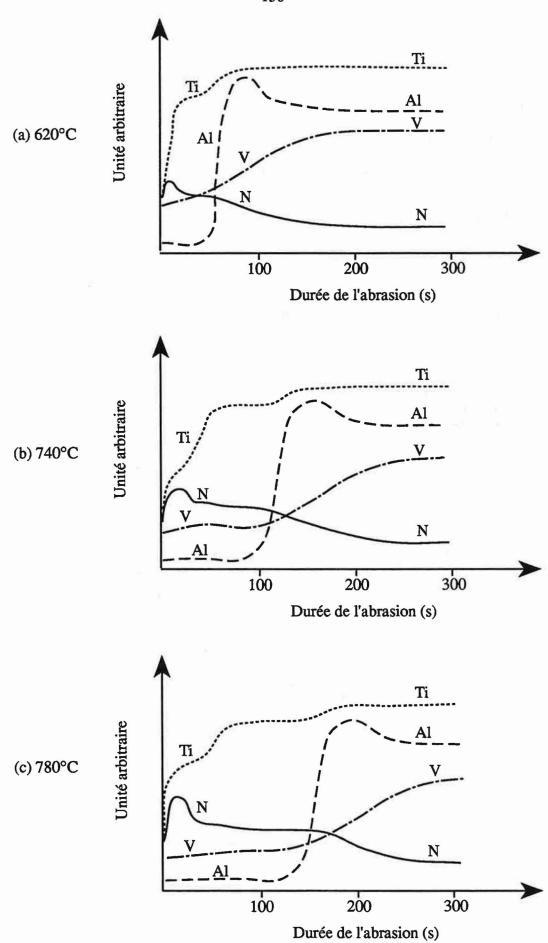
Figure 103 - Spectres SDL du TA6V nitruré - (a) 620°C; (b) 740°C; (c) 780°C
