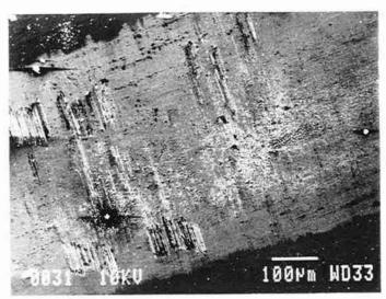
PMMA  $\Phi = 8 \text{ mm}$ TA6V = plan Force normale = 32 N Déplacement = ± 40 μm Fréquence = 1 Hz
