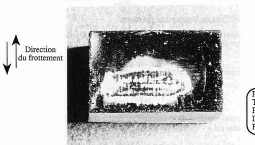
PMMA = plan TA6V = plan Force normale = 32 N Déplacement = ± 40 µm Fréquence = 1 Hz
