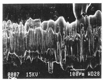
PMMA = plan TA6V = plan Force normale = 32 N Déplacement = ± 40 µm Fréquence = 1 Hz
