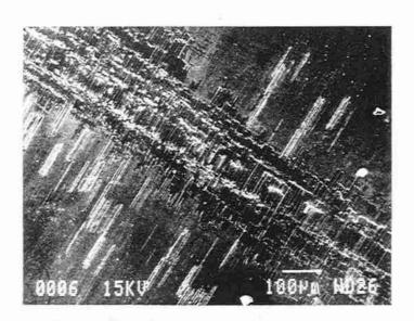
PMMA  $\Phi = 150 \text{ mm}$ TA6V = plan Force normale = 11 N Déplacement =  $\pm 40 \mu \text{m}$ Fréquence = 1 Hz
