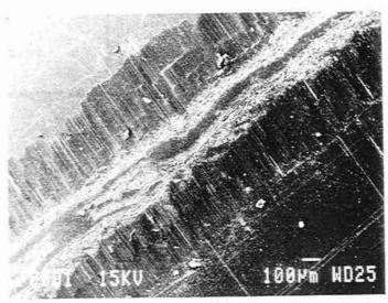
PMMA  $\Phi$  = 20 mm TA6V = plan Force normale = 300 N Déplacement =  $\pm$  60  $\mu$ m Fréquence = 1 Hz
