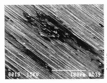
PMMA = plan 316L = planForce normale = 32 NDéplacement =  $\pm 40 \mu m$ Fréquence = 1 Hz
