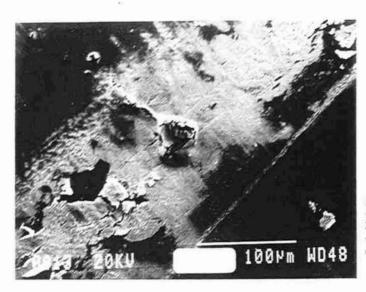
PMMA  $\Phi = 8 \text{ mm}$ TA6V = plan Force normale = 100 N Déplacement =  $\pm 40 \mu \text{m}$ Fréquence = 1 Hz
