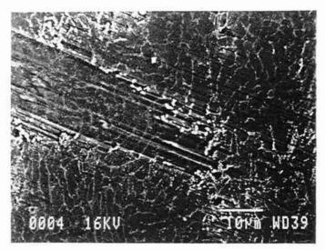
PMMA = plan TA6V impl. = plan Force normale = 32 N Déplacement = ± 40 µm Fréquence = 1 Hz
