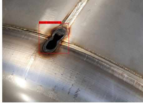
Figure 4.12: A defect detected by the model on an image of a different welding process.
